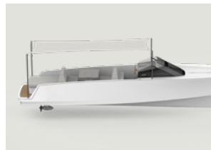
Removable sun awning with carbon fiber supports
