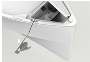
Anchor with electric windlass
