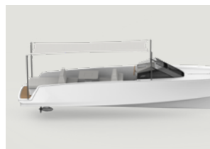
Removable sun awning with carbon fiber supports
